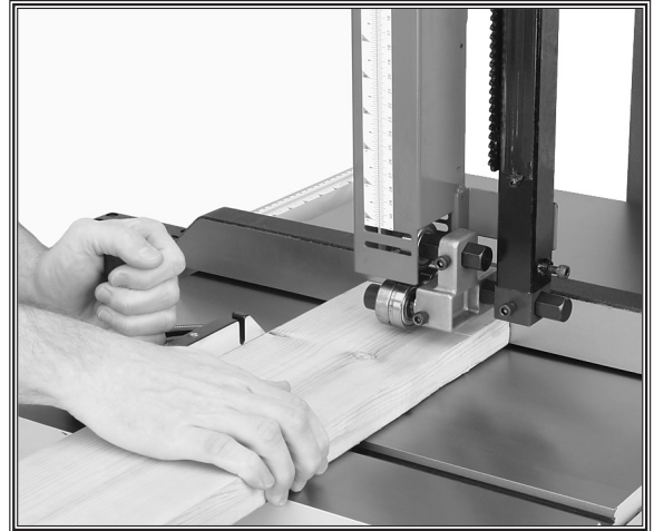
Figure 41. Typical crosscutting operation.
